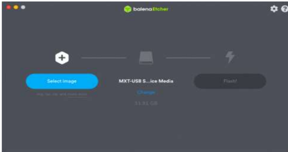
Figure 3.6: Flashing NVIDIA’s Jetpack image to a microSD card with balenaEtcher is one of the first steps for configuring your Nano for computer vision and deep learning.
